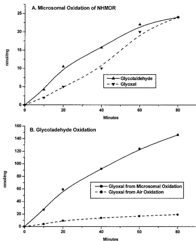
**Figure 4.** Yield of oxidation products from the microsomal oxidation of NDELA is shown as a function of time. Panel A shows that both glycolaldehyde and glyoxal are formed from the isoniazid induced microsomal oxidation of NHMOR at a substrate concentration of 0.4 mM. Panel B shows that glyoxal is formed from both the microsomal and nonenzymatic oxidation of glycolaldehyde (0.4 mM).
