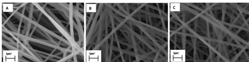
**Figure 6.** Morphology of electrospun neat SMA (A), SMA/Furanone 1 (B), and SMA/Furanone 2 nanofibers.
