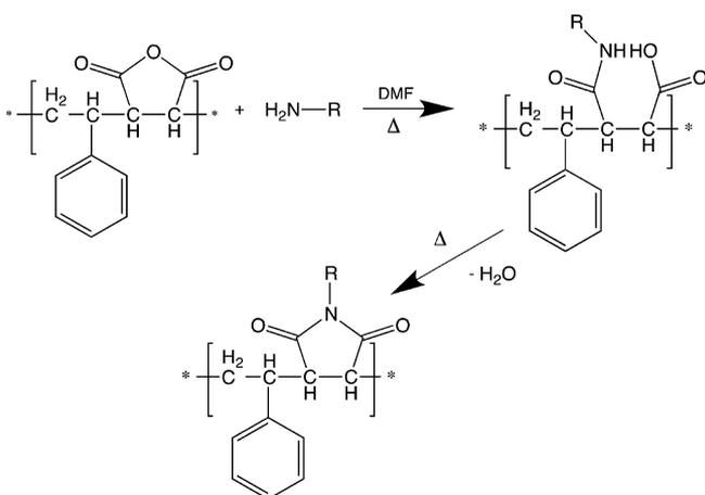
**Figure 3.** Immobilization of furanone derivatives on SMA copolymer backbone.<sup>39,41</sup>
