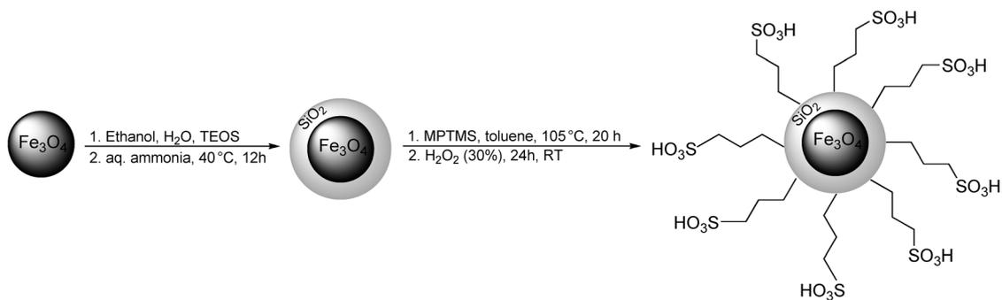
**Scheme 1.** Synthesis of sulfonated core-shell magnetic nanoparticles (SMNPs,  $\text{Fe}_3\text{O}_4@SiO_2@PrSO_3H$ ).
