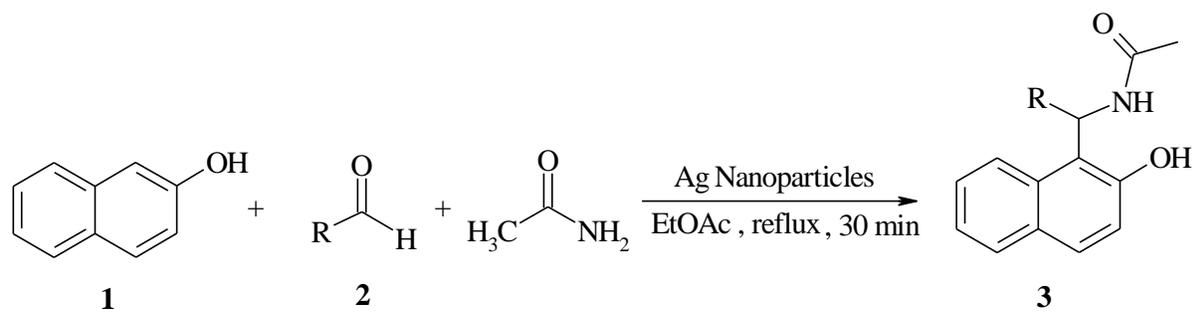
**Scheme 1:** Synthesis of 1-amidoalkyl-2-naphthols in the presence of silver NPs as catalyst
