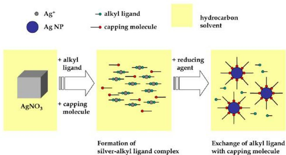
**Scheme 2:** Experimental schemes for direct synthesis of silver nanoparticles in fully organic phase through in situ ligand exchange
