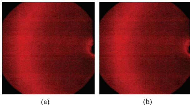
**FIGURE 1** X ray diffraction patterns of nonaligned samples of the (a) smectic chiral phase of [(L)Pd( $\mu$ -OAc)]<sub>2</sub> and (b) cholesteric phase of **1**.
