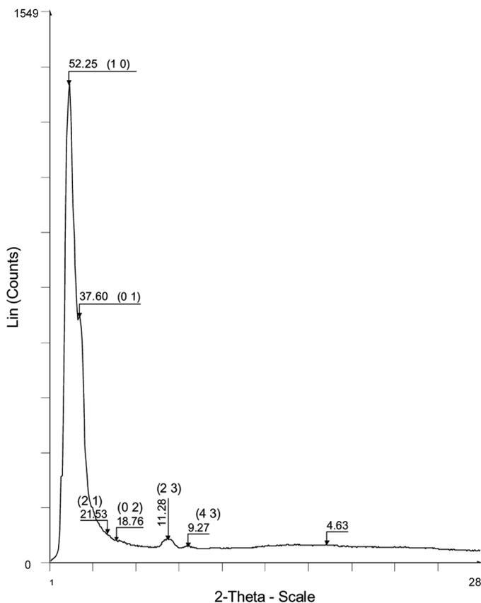
**FIGURE 2** X ray diffraction pattern of a non aligned sample of **2**, recorded at 180°C on cooling.
