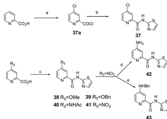
**Scheme 4.** Reagents and conditions: (a) SOCl<sub>2</sub>, DMF (cat.), 40–45 °C; (b) CH<sub>2</sub>Cl<sub>2</sub>, TEA, 2-aminothiazole; (c) 2-aminothiazole, DCC, HOBT, DMF; (d) DMF, NH<sub>3</sub> (g), 110 °C, 15%; (e) DMF, BnNH<sub>2</sub>, rt, 32%.
