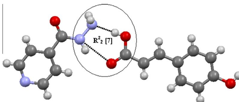
Fig. 2. Ring motif  $R_2^2 [7]$  in the cocrystal.
