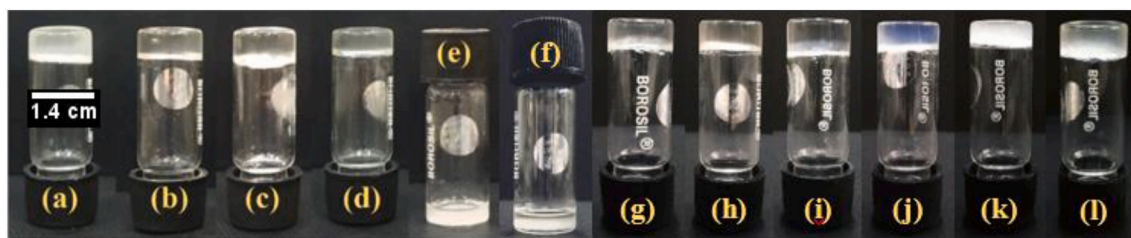
Fig. 4. Swelling studies of OG10 in (a) toluene, (b) THF, (c) chloroform, (d) 1,4-dioxane, (e) diethyl ether, (f) DMSO, (g) DMF, (h) DMAc, (i) 1,2-dichloroethane, (j) o-dichlorobenzene, (k) o-xylene, (l) ethyl acetate.
