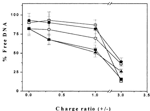
**Figure 2.** Percent of free DNA in lipid–DNA complexes prepared with four lipids (with cholesterol as colipid) and DOTAP. Agarose gels were scanned and quantitated by phosphorimager. By considering the total lane intensity as 100%, the free and complexed DNA percentages were calculated and replotted. Free DNA (percent) was plotted against charge ratio for lipids **1** (●), **2** (○), **3** (■), **4** (□), and DOTAP (▲) ( $n = 2$ ).
