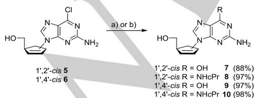
**Scheme 2.** Synthesis of CBV **9**, ABC **10** and their 1',2'-*cis*-analogues **7** and **8**. *Reagents and conditions:* for R = OH: a) 1 M aq. NaOH, reflux; for R = NHcPr: b) cyclopropylamine, EtOH, reflux.
