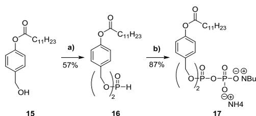
**Scheme 4.** Synthesis of the masked pyrophosphate **17**. *Reagents and conditions:* a) diphenyl phosphonate, pyridine, 40 °C; b) i) *N*-chlorosuccinimide, CH<sub>3</sub>CN, rt; ii) 0.4 M H<sub>2</sub>PO<sub>4</sub>NBu<sub>4</sub>, CH<sub>3</sub>CN, rt.
