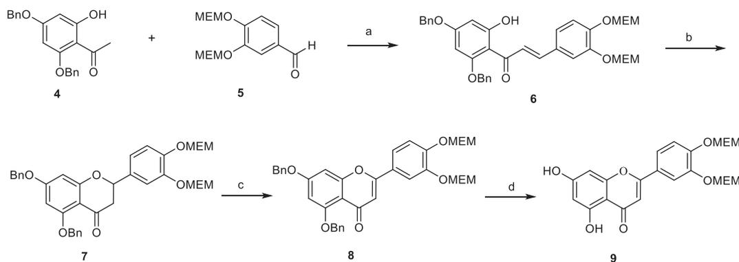
Scheme 1. Synthesis of intermediate **9**. Reagents and conditions: a. 20% KOH aq. ethanol, room temperature, 54%; b. NaOAc, H<sub>2</sub>O, ethanol, reflux, 46%; c. I<sub>2</sub>, pyridine, 100 °C, 69%; d. H<sub>2</sub>, Pd/C, EtOAc, room temperature, 85%.
