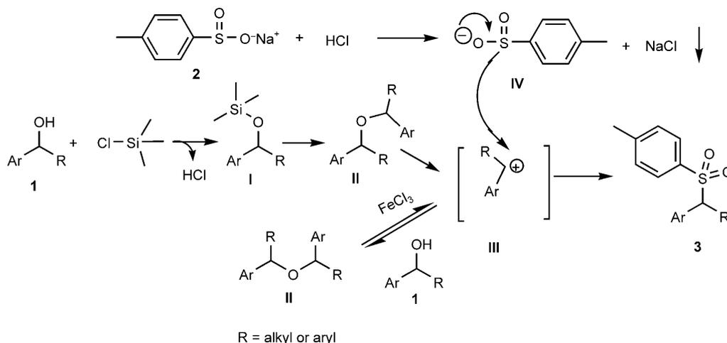
**Scheme 2.** Proposed mechanism for the direct sulfonylation of alcohols with sulfinate sodium salts using FeCl<sub>3</sub> and TMSCl.
