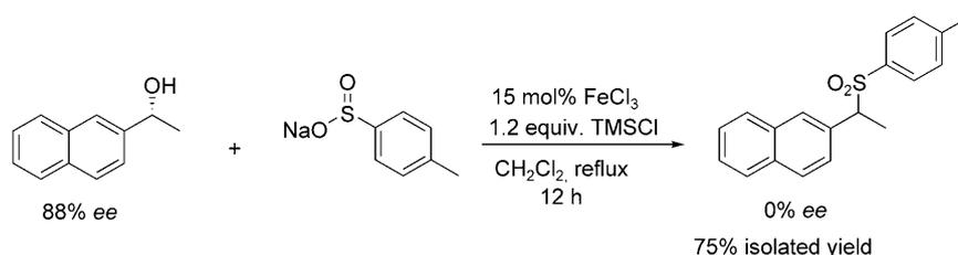
**Scheme 1.** Direct sulfonylation of an optically active alcohol with sodium *p*-toluenesulfinate salt.
