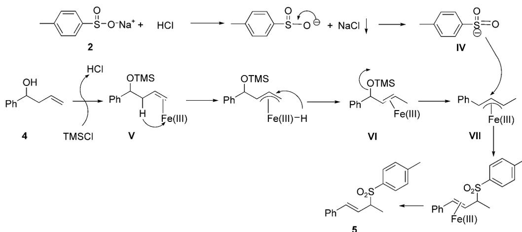
**Scheme 3.** Proposed mechanism for the direct sulfonylation of homoallylic alcohols with sodium *p*-toluenesulfonate using  $\text{FeCl}_3$  and TMSCl
