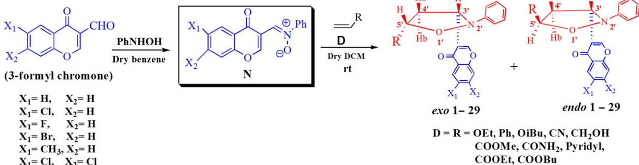
**Scheme 1:** Reaction of various nitrones (**N**) with monosubstituted dipolarophiles leads to chromanyl-isoxazolidines (**1-29**).
