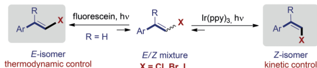
Scheme 1. Photocatalytic isomerization of functionalized alkenes.
