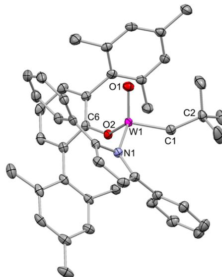
**Figure 1.** Thermal ellipsoid plot (50% probability) of  $W(O)(CH-t-Bu)(Ph_2Pyr)(OHMT)$  (**6**). Hydrogen atoms have been omitted for clarity. Selected bond distances (Å) and angles (deg):  $W1-C1 = 1.895(2)$ ,  $W1-O1 = 1.690(1)$ ,  $W1-O2 = 1.894(1)$ ,  $W1-N1 = 2.037(2)$ ;  $W1-C1-C2 = 141.1(1)$ ,  $W1-O2-C6 = 143.1(1)$ .
