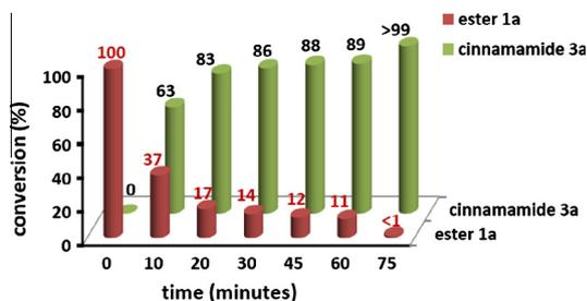
**Figure 3.** Reaction profile for amidation of ester **1a** with ethanolamine **2a** in the presence of  $\text{Na}_2\text{CO}_3$ .
