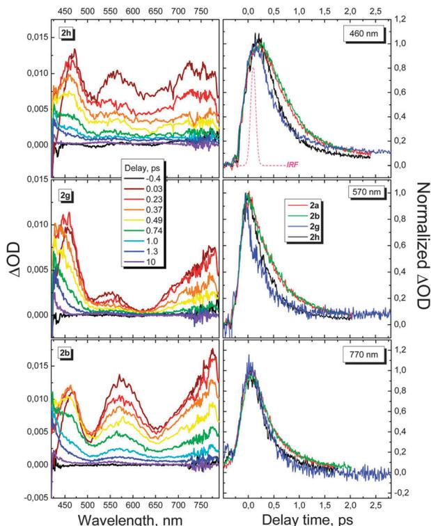
**Fig. 2** Left column: transient absorption spectra of GFP chromophores in MeCN after excitation at 370 nm. The  $-0.4$  ps trace corresponds to the spectral baseline in the absence of pump excitation. Right column: normalized kinetics of the TA signals. Color coding is the same for each column.
