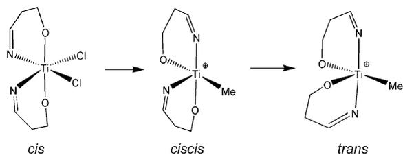
Scheme 2. Schematic representation of the plausible *cis* to *trans* change in complex configuration during the activation procedure. *cis* and *trans* abbreviations are related to the orientation of imine nitrogen atoms in complexes.
