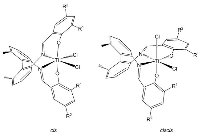
Scheme 3. The dimethylbiphenyl bridged titanium dichloride complexes (**1-Ti-3-Ti**) possess the *cis* or *ciscis* configuration or their combinations at room temp. in solution. **1-Ti** ( $R^1 = R^2 = H$ , *cis* and *ciscis* configurations in ratio of 1:4), **2-Ti** ( $R^1 = \textit{tert}$ -butyl,  $R^2 = H$ , *ciscis* configuration) and **3-Ti** ( $R^1 = R^2 = \textit{cumyl}$ , *cis* configuration).
