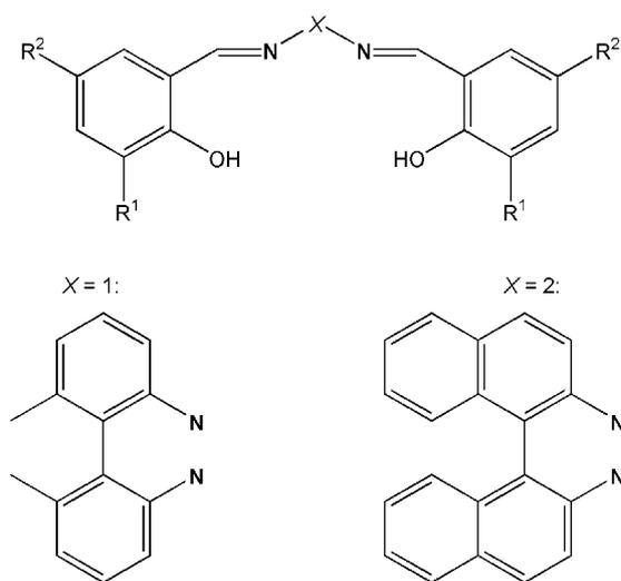
Scheme 7. Schematic representation of the biaryl-bridged salicylaldimine ligand precursors **1–4**. **1**:  $X = 1$ ,  $R^1 = R^2 = H$ ; **2**:  $X = 1$ ,  $R^1 = \textit{tert}$ -butyl,  $R^2 = H$ ; **3**:  $X = 1$ ,  $R^1 = R^2 = \text{CMe}_2\text{Ph}$ ; **4**:  $X = 2$ ,  $R^1 = \textit{tert}$ -butyl,  $R^2 = H$ .
