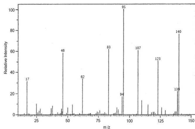
**Figure 2.** GC-mass spectrum of sulfoacetic acid with its molecular ion peak at 140 amu.
