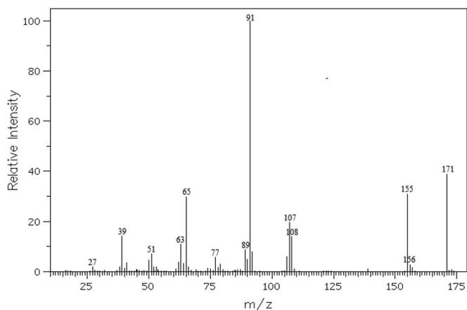
**Figure 1.** GC-mass spectra of p-toluenesulfonamide with its molecular ion peak at 171 amu.
