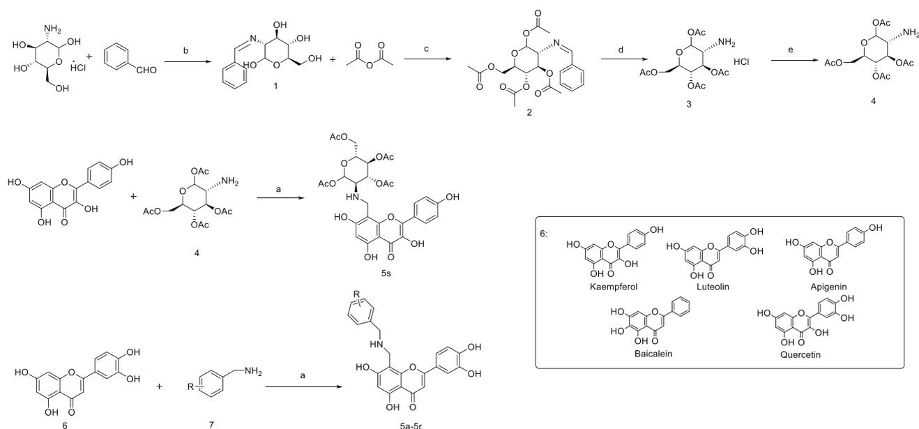
**Scheme 1** General synthesis of compounds **5a–5s**. Reagents and conditions: (a) HCHO (aq), isopropanol, 35 °C; (b) NaOH (aq), 0 °C; (c) pyridine, 40 °C, 6 h; (d) HCl, acetone, rt; (e) H<sub>2</sub>O, CH<sub>3</sub>COONa(aq), rt
