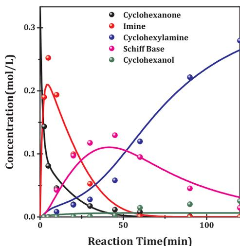
**Fig. 1.** Experimental (cycles) and modeled (solid lines) concentration of cyclohexanone and products in the reductive amination of cyclohexanone with methanol as solvent over Ru/C catalysts.
