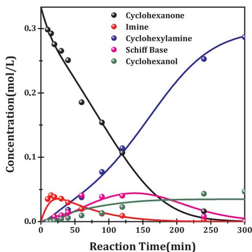
Fig. 4. Experimental (cycles) and modeled (solid lines) concentration of cyclohexanone and different products in the reductive amination of cyclohexanone with toluene as solvent over Ru/C catalyst.
