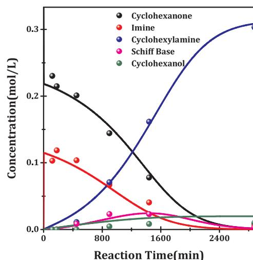
Fig. 5. Experimental (cycles) and modeled (solid lines) concentration of cyclohexanone and different products in the reductive amination of cyclohexanone with dioxane as solvent over Ru/C catalyst.
