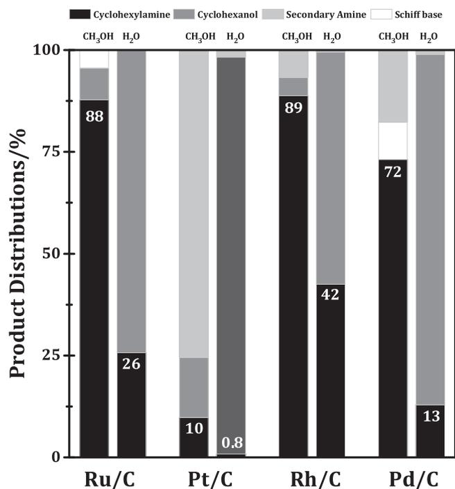
**Fig. 6.** Product distributions of reductive amination of cyclohexanone over Group VIII metal-based catalysts in methanol and water. Reaction conditions: Cyclohexanone 1 mmol, catalyst 0.02 g, solvent 3 mL, H<sub>2</sub> = 9 bar, T = 298 K, agitator speed = 1000 rpm, time = 2 h.
