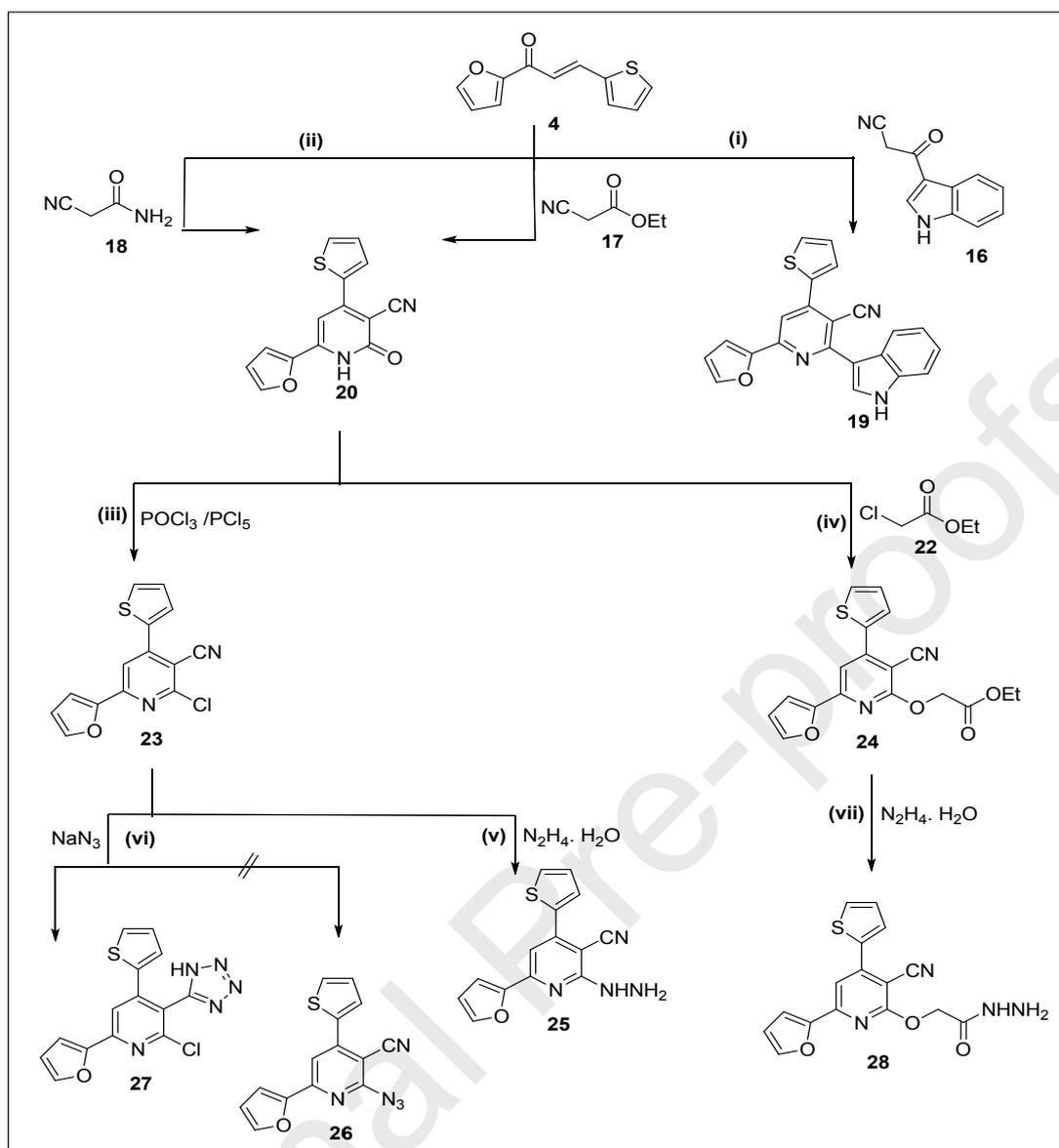
**Scheme 3** Reagents and conditions: (i)  $\text{NH}_4\text{OAc}$ , AcOH, reflux 12 h. (ii)  $\text{NH}_4\text{OAc}$ , n-butanol reflux 3h/ 5h. (iii) fusion at 80, 10 h. (iv)  $\text{K}_2\text{CO}_3$ , DMF, stirring, 24 h. (v) dioxane, reflux 12 h. (vi)  $\text{H}_2\text{O}$ , DMF, reflux 8 h. (vii) EtOH, reflux 7 h.
