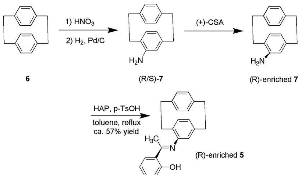
**Scheme 1.** Synthesis of (R)-5 from [2.2]paracyclophane (6). CSA, HAP, and p-TsOH stand for 10-camphorsulfonic acid, 2-hydroxyacetophenone, and *para*-toluenesulfonic acid, respectively.
