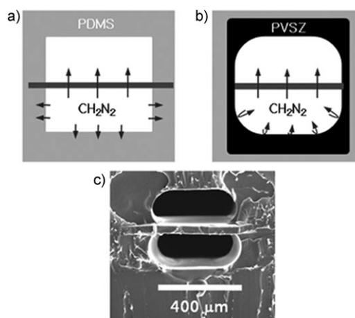
**Figure 2.** Restricted diffusion of  $\text{CH}_2\text{N}_2$  into the walls of a PDMS dual-channel reactor by PVSZ coating. a) Normal PDMS dual-channel reactor (unrestricted diffusion of  $\text{CH}_2\text{N}_2$ ); b) PVSZ-coated PDMS dual-channel (restricted diffusion of  $\text{CH}_2\text{N}_2$ ); c) cross-sectional SEM image of a typical PVSZ-coated PDMS dual-channel reactor.
