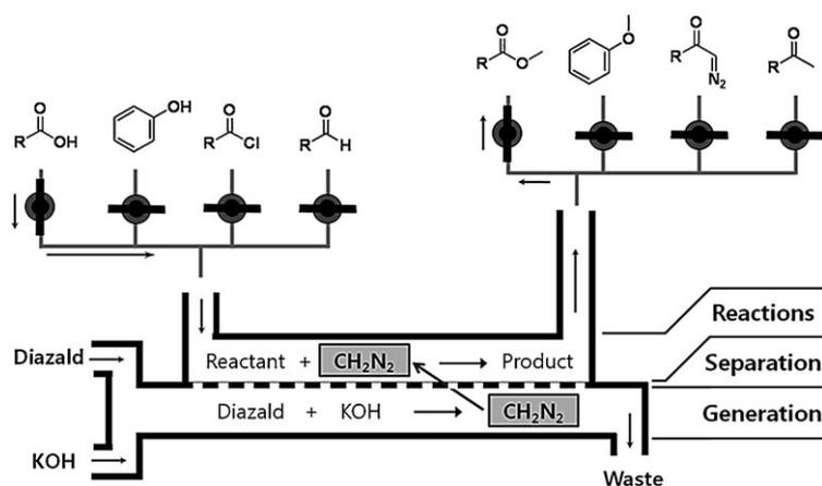
**Figure 1.** Illustration of the microchemical system for in-situ generation, separation, and reactions of diazomethane.
