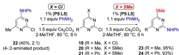
**Figure 2.** Selective palladium-catalyzed amination of substituted 2-chloro-4-thiomethoxy pyrimidines.
