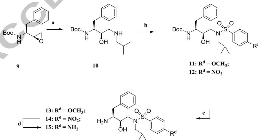
**Scheme 2.** Syntheses of amines **13-15**. Reagents and conditions: (a) *i*-BuNH<sub>2</sub>, CH<sub>3</sub>CN, 80 °C, 6 h; (b) Aryl sulfonyl chloride, DIEA, DMAP(Cat.), THF, 0 °C ~ r.t, 3- 5 h; (c) CH<sub>2</sub>Cl<sub>2</sub>-CF<sub>3</sub>COOH
