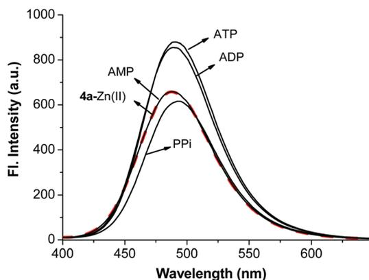
**Fig. 11** Fluorescence spectral change of **4a**-Zn(II) (10  $\mu$ M) in HEPES buffer (10 mM, pH 7.4; containing 1% CH<sub>3</sub>CN.  $\lambda_{\text{ex}} = 330$  nm) upon addition of anions (1 equiv.). PPi, ATP, ADP, and AMP were used as corresponding sodium salts.
