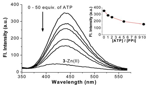
**Fig. 10** Influence of ATP on the fluorescence of **3**-Zn(II) (10  $\mu$ M) and PPi (50  $\mu$ M) in pH 7.4 buffer (10 mM HEPES containing 1% CH<sub>3</sub>CN): 0, 1, 2, 5, 10 equiv. of ATP with respect to PPi was added.  $\lambda_{\text{ex}} = 295$  nm. Inset: plot of the fluorescence intensity with respect to the molar ratio of [ATP]/[PPi].
