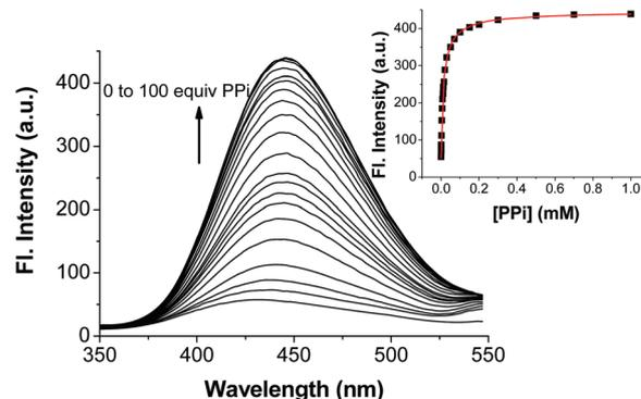
**Fig. 9** Fluorescence spectral change of **3**-Zn(II) (10  $\mu\text{M}$ ) upon gradual addition of PPi (0–1 mM) in pH 7.4 buffer (10 mM HEPES containing 1% CH<sub>3</sub>CN).  $\lambda_{\text{ex}} = 295$  nm. Inset: plot of fluorescence intensity vs. [PPi]. Due to the second-order diffraction interference at 570 nm, the fluorescence data were cut down at 550 nm.
