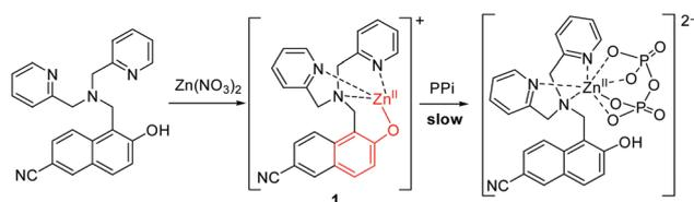
Fig. 1 Aryloxy-Zn(DPA) **1** and its binding mode with PPi.
