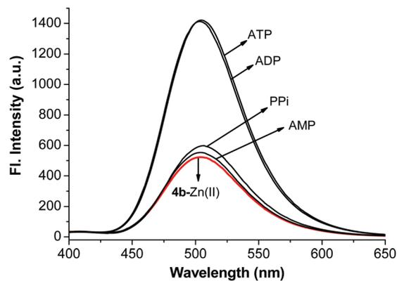
**Fig. 12** Fluorescence spectral change of **4b**-Zn(II) (10  $\mu$ M) in pH 7.4 buffer (10 mM HEPES containing 1% CH<sub>3</sub>CN) upon addition of anions (1 equiv.).  $\lambda_{\text{ex}} = 370$  nm. PPi, ATP, ADP, and MP were used as corresponding sodium salts.
