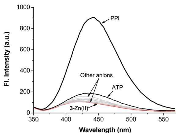
**Fig. 7** Fluorescence spectral change of **3**-Zn(II) (10  $\mu\text{M}$ ) (the bottom red line) upon addition of each of various anions (5 equiv.; F<sup>-</sup>, Cl<sup>-</sup>, OH<sup>-</sup>, CN<sup>-</sup>, CH<sub>3</sub>COO<sup>-</sup>, HSO<sub>4</sub><sup>-</sup>, HPO<sub>4</sub><sup>-</sup>, PO<sub>4</sub><sup>-</sup>, AMP, ADP, ATP and PPi; as sodium salts, except KF) in pH 7.4 buffer (10 mM HEPES containing 1% CH<sub>3</sub>CN).  $\lambda_{\text{ex}} = 295$  nm.
