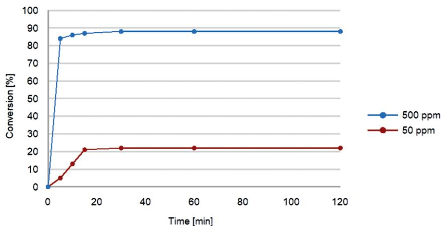
Figure 5. Activity of **[Ru-12]** in the model RCM reaction of **S1**.
