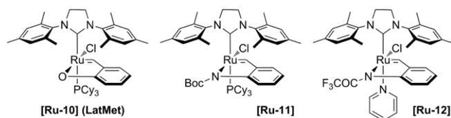
Figure 2. Our previously synthesised latent Ru catalysts bearing anionic benzylidene ligands.
