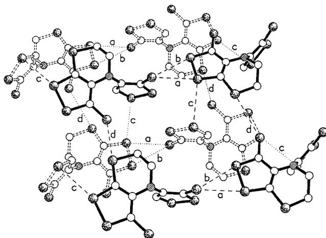
**Figure 4.** Part of two overlapping sheets of molecules of **5** showing the *intra* and *intersheet* S...S interactions. The S...S distances (Å) are (a) 3.31; (b) 3.45; (c) 3.52; (d) 3.55.
