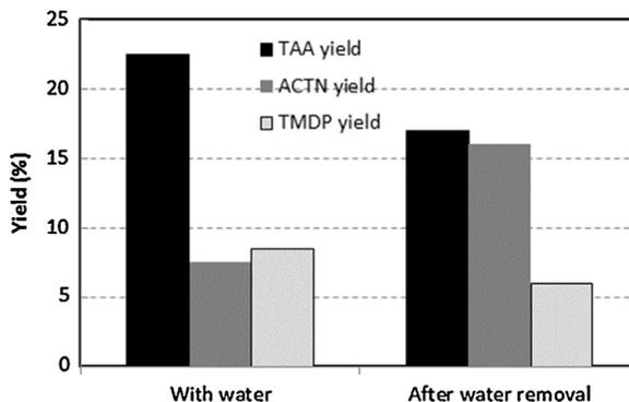
**Fig. 4.** Effect of water removal by anhydrous sodium sulfate in the presence of NH<sub>4</sub>Cl catalyst. Reaction conditions: *T* 65 °C, acetone/ammonia mol. ratio 4.0, catalyst/acetone wt ratio 0.02, and reaction time 6 h.
