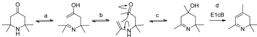
**Scheme 4.** An hypothesis about the mechanism for the irreversible transformation of TAA into TMDP.
