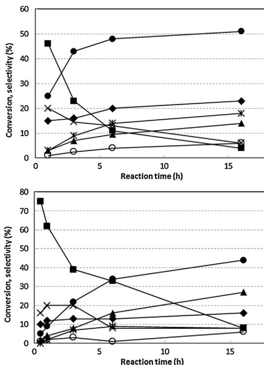
**Fig. 7.** Acetone conversion and selectivity to products as functions of time with HY-6 (Top) and HY-200 (Bottom) zeolites. Reaction conditions: acetone/ammonia mol. ratio 10.0, catalyst/acetone wt ratio 0.10, T 65 °C. Symbols: (◆) Acetone conversion (%). Selectivity (%) to: (●) TAA, (■) ACTN, (▲) TMDP, (○) DAA, (✱) MO, and (✕) DAAM.
