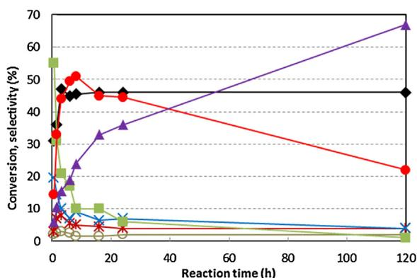
**Fig. 1.** Acetone conversion and selectivity to products in the presence of  $\text{NH}_4\text{Cl}$  catalyst in function of reaction time. Reaction conditions: acetone/ammonia mol. ratio 4.0, catalyst/acetone wt ratio 0.02,  $T$  65 °C. Symbols: (◆) Acetone conversion (%). Selectivity (%) to: (●) TAA, (■) ACTN, (▲) TMDP, (○) DAA, (✱) MO, and (×) DAAM.
