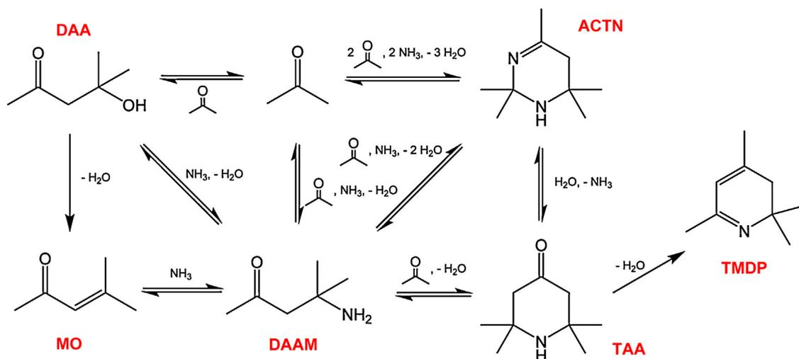
**Scheme 5.** Reaction scheme of TAA synthesis by direct reaction between acetone and ammonia.
