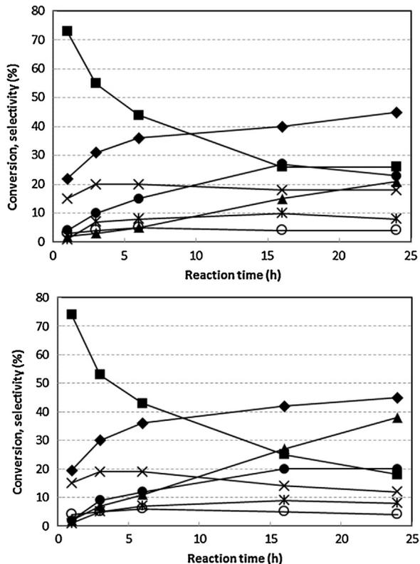
**Fig. 6.** Acetone conversion and selectivity to products in the presence of HY-6 (top) and HY-200 (bottom) zeolites in function of reaction time. Reaction conditions: acetone/ammonia mol. ratio 4.0, catalyst/acetone wt ratio 0.10, T 65 °C. Symbols: (◆) Acetone conversion (%). Selectivity (%) to: (●) TAA, (■) ACTN, (▲) TMDP, (○) DAA, (✱) MO, and (✕) DAAM.
