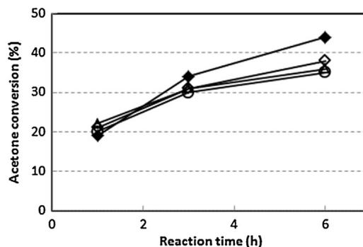
**Fig. 5.** Acetone conversion in function of reaction time. Symbols: catalyst HY-6 ( $\Delta$ ), HY-15 ( $\diamond$ ), HY-200 ( $\circ$ ), and  $\text{NH}_4\text{Y-15}$  ( $\blacklozenge$ ). Reaction conditions: acetone/ammonia mol. ratio 4.0, catalyst/acetone wt ratio 0.10, T 65 °C.
