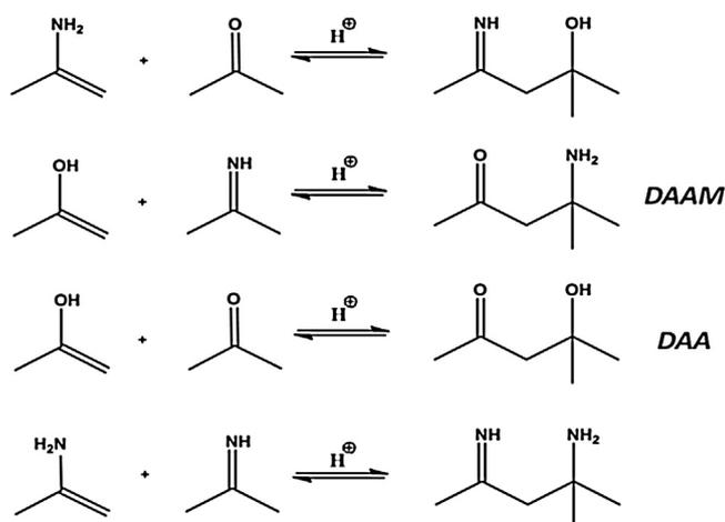
**Scheme 6.** Aldol condensation of acetone and dimethylketimine (or the corresponding enolic forms).
