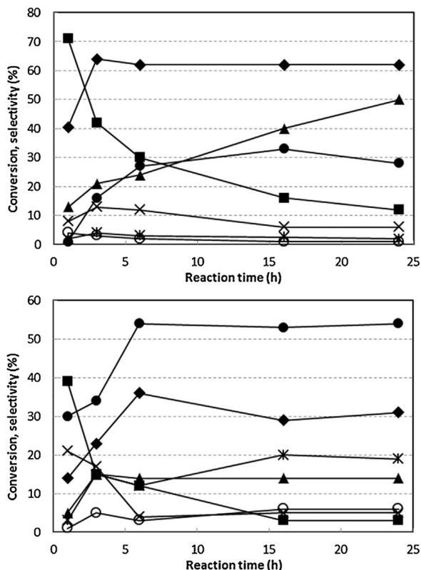
**Fig. 2.** Acetone conversion and selectivity to products in the presence of NH<sub>4</sub>Cl catalyst and with different acetone/ammonia molar ratios in function of reaction time. Top: acetone/ammonia mol. ratio 2.5. Bottom: acetone/ammonia mol. ratio 10.0. Reaction conditions: *T* 65 °C, catalyst/acetone wt ratio 0.02. Symbols: (◆) Acetone conversion (%). Selectivity (%) to: (●) TAA, (■) ACTN, (▲) TMDP, (○) DAA, (✱) MO, and (×) DAAM.
