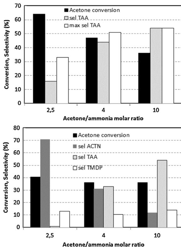
**Fig. 3.** Comparison of catalytic behaviour for different acetone/ammonia molar ratios at the maximum acetone and ammonia conversion (top), and for similar acetone conversions (bottom), in the presence of NH<sub>4</sub>Cl catalyst. Other conditions as in Figs. 1 and 2.
