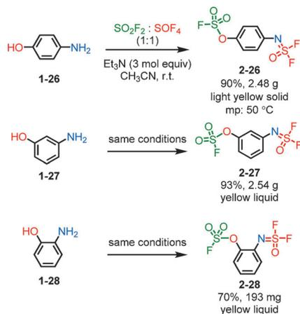
**Figure 3.** The selectivity of  $\text{SO}_2\text{F}_2$  and  $\text{SOF}_4$  towards aromatic hydroxy and amino groups.
