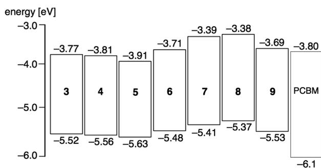
Figure 2. HOMO–LUMO levels of 3–9, with PCBM included as a reference.
