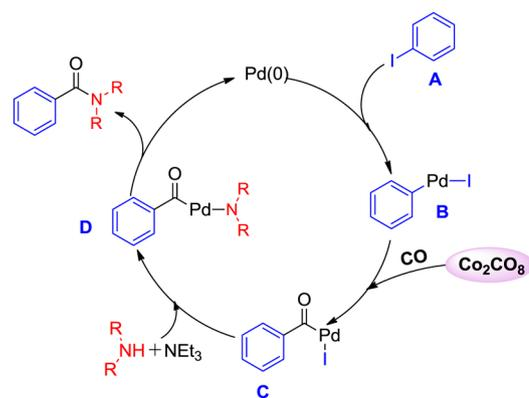
**Fig. 2.** Plausible reaction mechanism of the Aminocarbonylation reaction.
