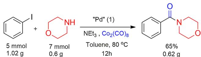
**Scheme 1.** Palladium catalyzed gram scale synthesis of esters using Co<sub>2</sub>(CO)<sub>8</sub> as C1 source.
