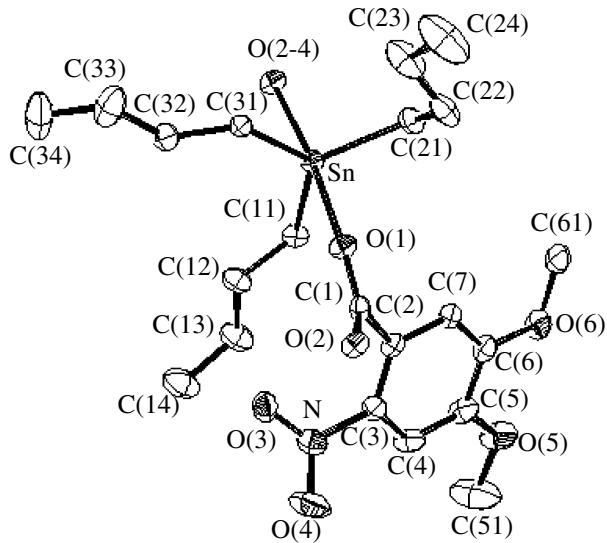
**Fig. 2.** Refined ORTEP drawing of the X-ray structure of compound **II**.
