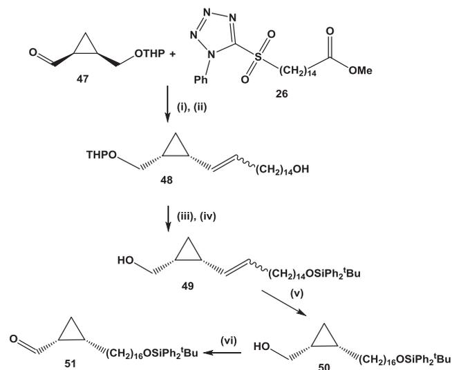
**Scheme 13.** (i) LiBSA, THF,  $-10$  °C (89%); (ii)  $\text{LiAlH}_4$ , THF (80%); (iii)  $^t\text{BuPh}_2\text{SiCl}$ ,  $\text{Et}_3\text{N}$ ,  $\text{CH}_2\text{Cl}_2$  (95%); (iv) PPTS, MeOH/THF  $50$  °C (82%); (v)  $\text{KO}_2\text{CN}=\text{NCO}_2\text{K}$ , AcOH, THF, MeOH (98%); (vi) PCC,  $\text{CH}_2\text{Cl}_2$  (98%).
