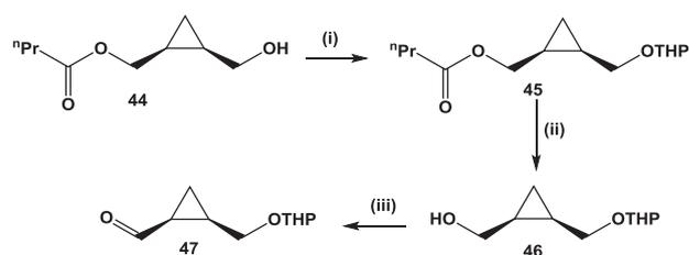
**Scheme 12.** (i) PPTS,  $\text{CH}_2\text{Cl}_2$ , 3,4-dihydro-2H-pyran (84%); (ii)  $\text{LiAlH}_4$ , THF (92%); (iii) PCC,  $\text{CH}_2\text{Cl}_2$  (54%).
