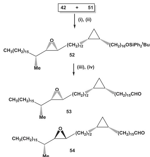
**Scheme 14.** (i) LiBSA, THF,  $-10$  °C (89%); (ii)  $\text{KO}_2\text{CN}=\text{NCO}_2\text{K}$ , AcOH, THF, MeOH (80%); (iii) TBAF, THF (91%); (iv) PCC,  $\text{CH}_2\text{Cl}_2$  (76%).
