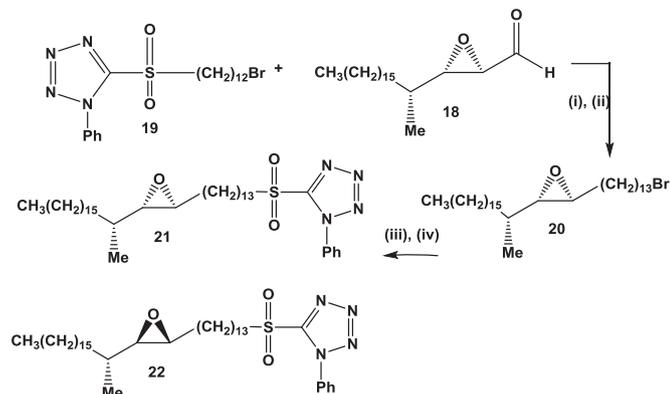
**Scheme 6.** (i) LiBSA, THF,  $-10$  °C (71%); (ii)  $\text{KO}_2\text{CN}=\text{NCO}_2\text{K}$ , AcOH, THF, MeOH (93%); (iii) 1-phenyl-1*H*-tetrazole-5-thiol, acetone,  $\text{K}_2\text{CO}_3$  (82%); (iv)  $\text{H}_2\text{O}_2$ ,  $\text{Mo}_7\text{O}_{24}(\text{NH}_4)_6 \cdot 4\text{H}_2\text{O}$ , IMS (industrial methylated spirit), THF (67%).
