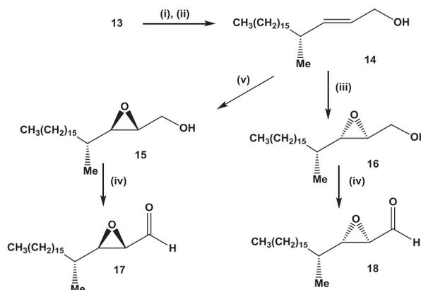
Scheme 5. (i) Ph<sub>3</sub>P=CHCOOMe, toluene (65%); (ii) DIBAL, CH<sub>2</sub>Cl<sub>2</sub> (95%); (iii) L-(+)-diethyl tartrate, Ti(Oi-Pr)<sub>4</sub>, *t*-BuOOH, CH<sub>2</sub>Cl<sub>2</sub>, –20 °C (75%); (iv) PCC, CH<sub>2</sub>Cl<sub>2</sub> (59% **18**), (60% **17**); (v) D-(–)-diethyl tartrate, Ti(Oi-Pr)<sub>4</sub>, *t*-BuOOH, CH<sub>2</sub>Cl<sub>2</sub>, –20 °C (67%).
