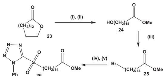
**Scheme 7.** (i) NaOMe, MeOH; (ii)  $\text{H}_2\text{SO}_4$ , MeOH, reflux (85% for two steps) (iii)  $\text{Ph}_3\text{P}$ , NBS,  $\text{NaHCO}_3$ ,  $\text{CH}_2\text{Cl}_2$  (88%) (iv) 1-phenyl-1*H*-tetrazole-5-thiol,  $\text{K}_2\text{CO}_3$ , acetone (90%); (v)  $\text{Mo}_7\text{O}_{24}(\text{NH}_4)_6 \cdot 4\text{H}_2\text{O}$ ,  $\text{H}_2\text{O}_2$ , THF/IMS (91%).
