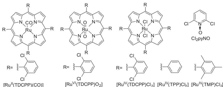
**Scheme 1.** Ruthenium porphyrin catalysts and oxidant Cl<sub>2</sub>pyNO.
