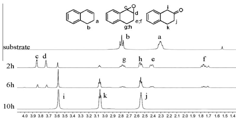
**Figure 1.**  $^1\text{H}$  NMR of oxidation of benzocyclohexene with  $\text{Cl}_2\text{pyNO}$  catalyzed by  $[\text{Ru}^{\text{IV}}(\text{TDCPP})\text{Cl}_2]$  changed over time.
