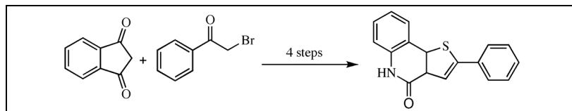
2-Phenacylindan-1,3-dione (**3**) was treated with Lawesson's reagent (2,4-bis(4-methoxyphenyl)-1,3-dithia-2,4-diphosphetane-2,4-disulfide) to form 2-phenyl-4*H*-indeno[1,2-*b*]thiophene-4-one (**4**). Compound **4** was subsequently reacted with hydroxyl amine to form the oxime (**5**), which, upon treatment with polyphosphoric acid, underwent ring expansion (Beckmann rearrangement) to give 2-phenylthieno[3,2-*c*]quinoline-4(5*H*)-one.
