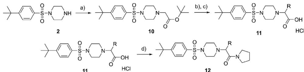
**Scheme 4.** Synthesis to yield compounds with mono-substitution alpha to the carboxamide. *Reagents and conditions:* (a) tert-butyl bromoacetate; (b) LiHMDS, RI or RBr, THF, –78 °C – 24 °C. K<sub>2</sub>CO<sub>3</sub>, ACN, reflux; (c) 4 M HCl, dioxane, 90 °C; (d) HBTU, pyrrolidine, DMF, 24 °C.
