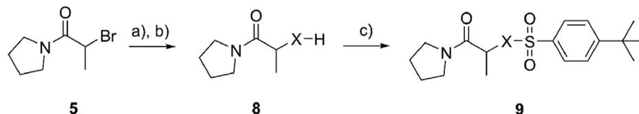
**Scheme 3.** Synthetic pathway to yield analogues incorporating piperazine variations or isosteres. *Reagents and conditions:* (a) Boc-X-H, DIPEA, EtOH, 70 °C; (b) TFA/DCM, 20 °C; (c) 4-tert-butylbenzenesulfonyl chloride, DIPEA, DCM, 40 °C.
