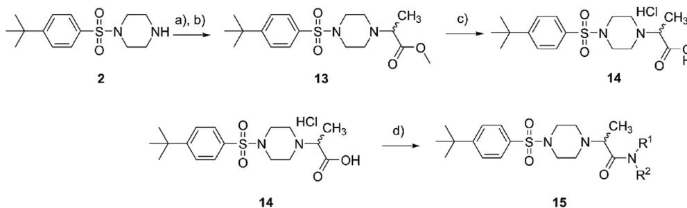
**Scheme 5.** Synthetic pathway to afford enantiopure analogues. *Reagents and conditions:* (a) methyl (R)-(+)-lactate or methyl (S)-(-)-lactate, triflic anhydride, 2,6-lutidine, DCM, -78 °C – 24 °C; (b) 1-((4-*tert*-butyl)phenyl)sulfonyl piperazine (**2**), DCM, 0 °C–24 °C; (c) 4 M HCl, dioxane, 90 °C; (d) HBTU, NHR<sup>1</sup>R<sup>2</sup>, DMF, 24 °C.
