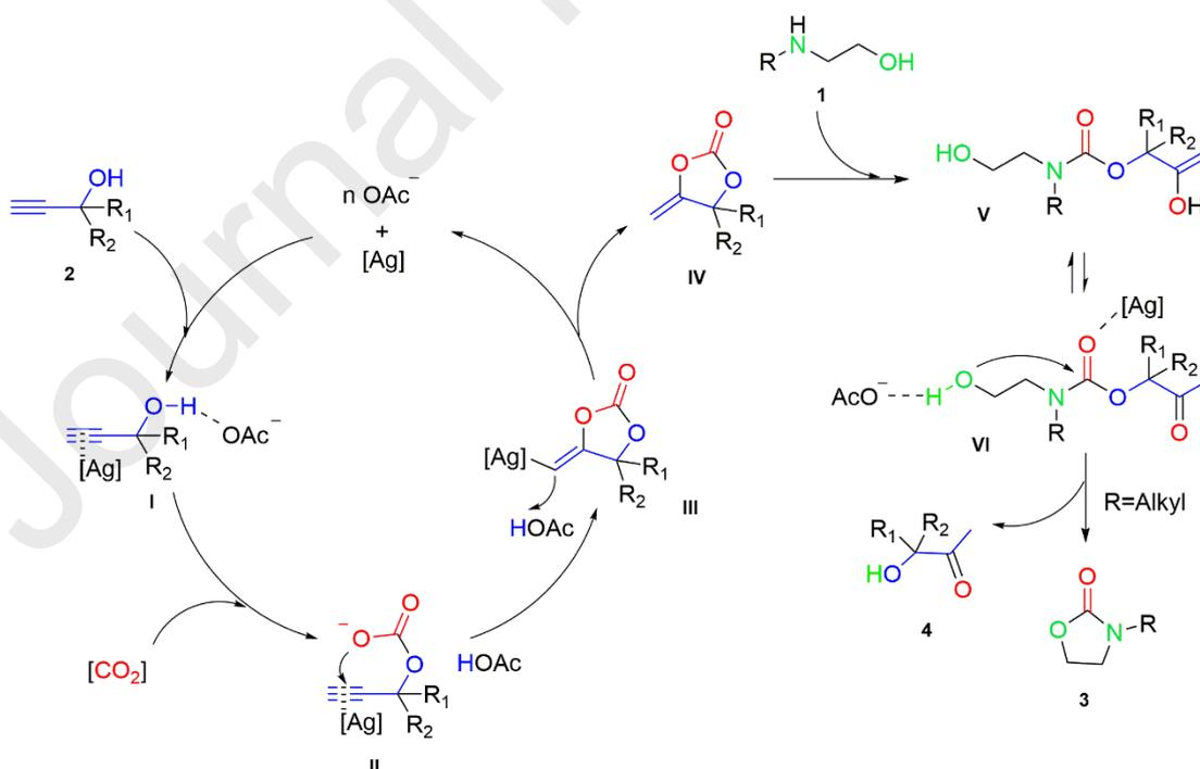
**Scheme 1.** Proposed catalytic mechanism of the  $\text{AgNO}_3/[\text{C}_2\text{C}_1\text{im}][\text{OAc}]$  system.
