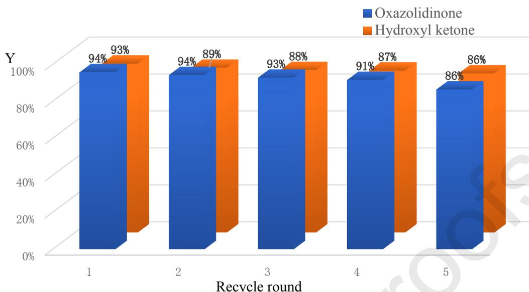
**Fig. 1.** Reusability of the  $\text{AgNO}_3/[\text{C}_2\text{C}_1\text{im}][\text{OAc}]$  system.
