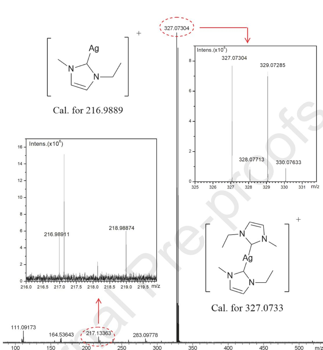
**Fig. 6.** Detection of the NHC-Ag complexes during the catalytic process.
