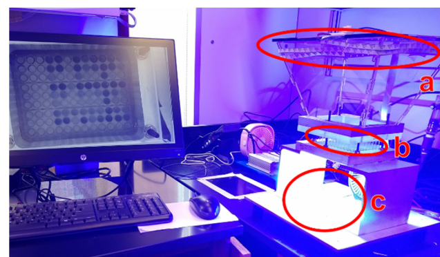
Figure 2. (a) White LED strips and camera attached to a plexiglass cage for monitoring reaction progress; (b) 108 reaction vials (1 mL) covered in H 2 -sensitive colorimetric tape sealed with silicone and plexiglass; (c) two 100 W blue LED chips (440 ± 10 nm).
