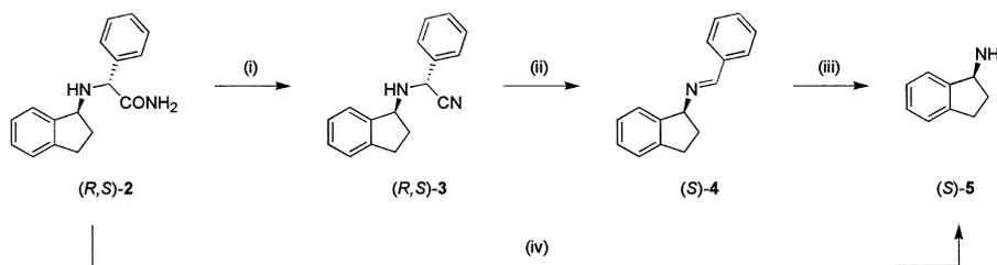
**Scheme 2.** Non-reductive chiral auxiliary removal furnishing (*S*)-**5**. *Reagents and conditions:* (i) POCl<sub>3</sub>, Et<sub>3</sub>N, CH<sub>2</sub>Cl<sub>2</sub>, 0°C→rt, 1 h; (ii) K<sub>2</sub>CO<sub>3</sub>, EtOH, reflux, 1 h; (iii) NH<sub>2</sub>OH·HCl, THF/H<sub>2</sub>O 1:1, 20 h; (iv) POCl<sub>3</sub>, Et<sub>3</sub>N, THF, 0°C→reflux, 5 h; NH<sub>2</sub>OH·HCl, H<sub>2</sub>O, 16 h.
