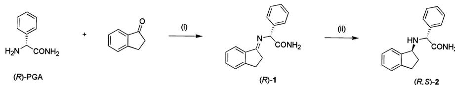
**Scheme 1.** Synthesis of amine (*R,S*)-2. Reagents and conditions: (i) *p*-TsOH·H<sub>2</sub>O, *i*-PrOAc, reflux, ca. 6 h; (ii) Ra-Ni, 3.5 bar H<sub>2</sub>, 40°C, 45 h.
