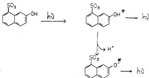
Figure 1. Schematic depiction of 2-naphthol-8-sulfonate excited-state proton transfer.
