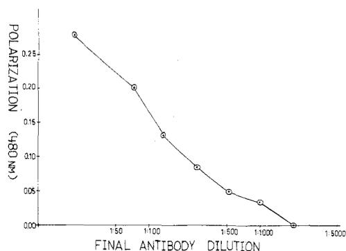
**Figure 3.** Variation in fluorescence polarization of  $7.5 \times 10^{-7}$  M 2-8-DPH with varying dilutions of rabbit anti-DPH.
