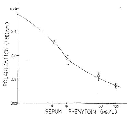
**Figure 4.** Fluorescence polarization immunoassay standard curve illustrating the change in polarization of 2-8-DPH with increasing concentrations of unlabeled phenytoin.**Table II. Precision of Phenytoin Analysis by FPIA<sup>a</sup>**
