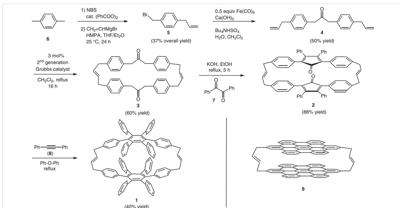
**Scheme 1** Synthesis of 2,24-diene-12,13,15,16,34,35,37,38-octaphenyl[4.4]triphenylparacyclophane (**1**)
