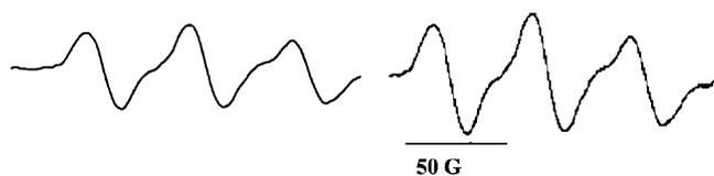
**Figure 2.** ESR spectroscopy of the radical released by **C1** and **C6**. ESR with PBN (*N-tert-butyl- $\alpha$ -phenylnitrone*) trapping in benzene under light. Microwave frequency 9.782 GHz, mid range 3430 G, scan range.
