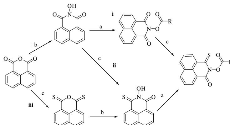
**Scheme 2.** Reagents and conditions: (a)  $\text{RCOCl}$ ,  $\text{NEt}_3$ , rt, 45 min; (b)  $\text{NH}_2\text{OH}\cdot\text{HCl}$ ,  $\text{NEt}_3$ ,  $\text{CH}_3\text{CH}$ , reflux, 2 h; (c) Lawesson's reagent,  $\text{C}_6\text{H}_5\text{-Cl-}p$ , reflux, 1 h.
