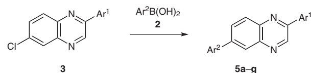
Scheme 3 Synthesis of 5a–g . Reagents and conditions: 3 (1 equiv), 2 (1.3 equiv), Pd(PPh 3 ) 4 (5 mol%), 2 M K 2 CO 3 , 1,4-dioxane, 120 °C, 8 h.
