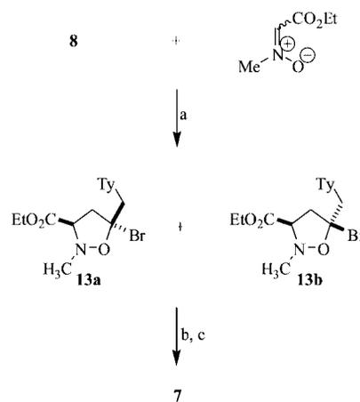
Scheme 3. a) THF, microwave at 300 W, 80 °C, 3 h; b) NaBH<sub>4</sub>, MeOH; c) Et<sub>3</sub>N.
