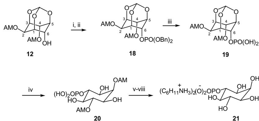
**Scheme 3.** Reagents and conditions: (i)  $(\text{BnO})_2\text{PN}(i\text{-Pr})_2$ , tetrazole,  $\text{CH}_2\text{Cl}_2$ ,  $-42^\circ\text{C}$ ; (ii) *m*-CPBA,  $-78^\circ\text{C}$ , 90%; (iii)  $\text{H}_2$ , 5% Pd/C, EtOAc; (iv) TFA– $\text{H}_2\text{O}$ , rt, 12 h; (v) 1 M LiOH, THF, rt, 12 h; (vi)  $\text{H}^+$ , extract with  $\text{CH}_2\text{Cl}_2$ ; (vii) DIAION SK1BH ( $\text{H}^+$  form) resin; (viii)  $\text{C}_6\text{H}_{11}\text{NH}_2$ , rt, 10 min.
