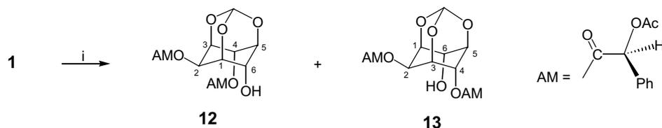
**Scheme 1.** Reagents and conditions: (i) (*S*)-(+)-*O*-acetylmandeloyl chloride (2.1 equiv), py, 0 °C, 2 h.
