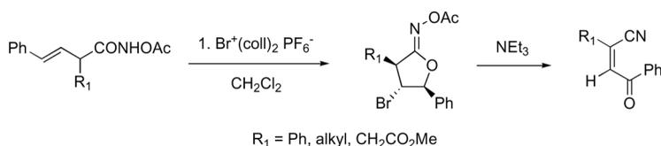
**Abstract** Reaction of  $\gamma$ -phenyl- $\beta,\gamma$ -unsaturated hydroxamates with bis(collidine)-bromine(I) hexafluorophosphate led to the formation of cyclic bromo imidates. Reaction of these with triethylamine led to the formation of 3-cyano-2-propen-1-ones with good yields by a fragmentation reaction.
