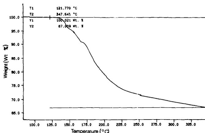
**Figure 4—Thermogravimetric analysis of trimelamol (1) at a rate of 5.0 °C/min.**
