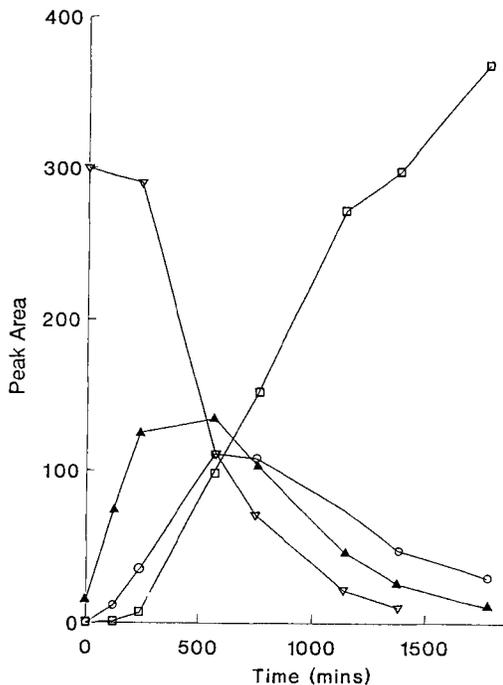
**Figure 3**—Plot of relative concentrations of trimelamol (1) and all degradation products versus time at pH 7.4 and 37 °C. Key: (▽) 1; (▲) 2; (○) 3; (□) 4.
