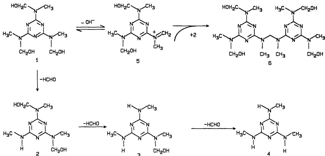
Scheme 1—Degradation pathways of trimelamol (1) in aqueous solution.
