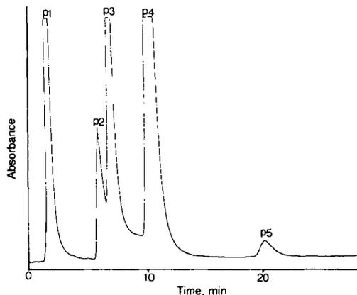
**Figure 6**—Analytical HPLC trace of the lyophilizate from preparative HPLC. Peaks are numbered in order of elution: P1 = DMSO (solvent); P2 = N<sup>2</sup>,N<sup>4</sup>,N<sup>6</sup>-trimethylmelamine (4); P3 = N<sup>2</sup>-monomethylol-N<sup>2</sup>,N<sup>4</sup>,N<sup>6</sup>-trimethylmelamine (3); P4 = N<sup>2</sup>,N<sup>4</sup>-dimethylol-N<sup>2</sup>,N<sup>4</sup>,N<sup>6</sup>-trimethylmelamine (2); and P5 = trimelamol (1).
