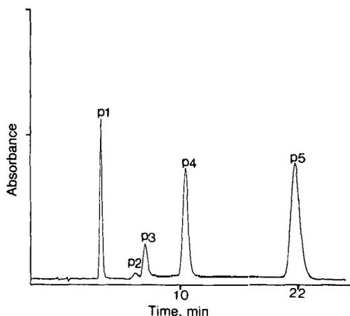
Figure 1—Typical HPLC chromatogram of trimelamol (1) undergoing degradation in aqueous solution. Peaks are numbered in order of elution: P1 = resorcinol (internal standard); P2 = *N*<sup>2</sup>,*N*<sup>4</sup>,*N*<sup>6</sup>-trimethylmelamine (4); P3 = *N*<sup>2</sup>-monomethylol-*N*<sup>2</sup>,*N*<sup>4</sup>,*N*<sup>6</sup>-trimethylmelamine (3); P4 = *N*<sup>2</sup>,*N*<sup>4</sup>-dimethylol-*N*<sup>2</sup>,*N*<sup>4</sup>,*N*<sup>6</sup>-trimethylmelamine (2); and P5 = trimelamol (1).
