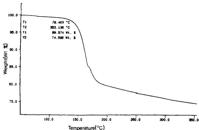
**Figure 5**—Thermogravimetric analysis of bis(trimelamol) (6) at a rate of 5.0 °C/min.
