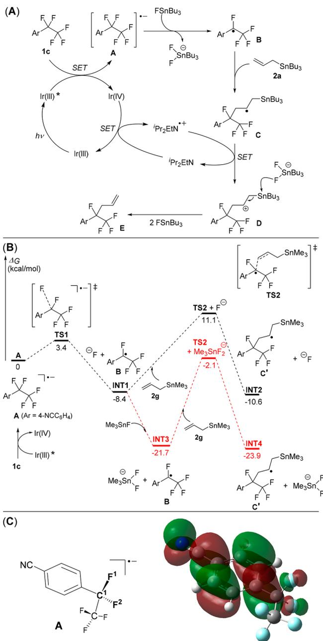
**Figure 3.** (A) Plausible mechanism for photoredox-catalyzed defluoroallylation of **1c** with **2a**. (B) Free energy profile for tin fluoride-accelerated defluoroallylation. (C) SOMO of radical anion **A**.
