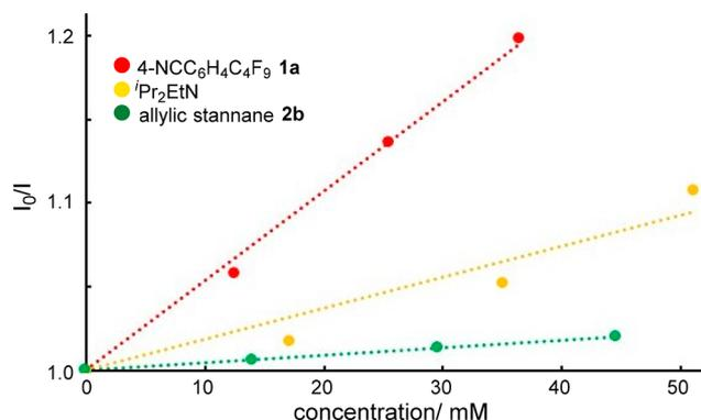
**Figure 2.** Stern–Volmer luminescence quenching studies of photocatalyst Ir(ppy)<sub>3</sub> (excitation 380 nm, emission 514 nm).
